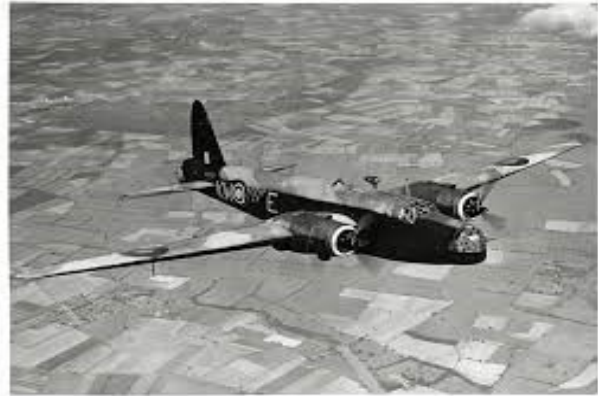
A Vickers Wellington BMkIII, powered by Bristol Hercules engines and with a four-gun tail turret
