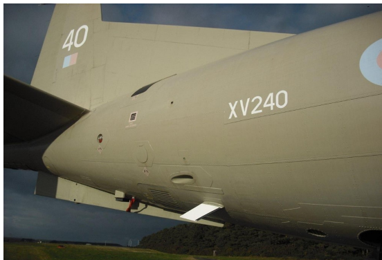
Extra ventral fin on the Nimrod to improve stability
